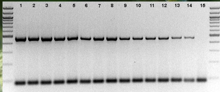
Fig.3. Example of electrophoresis gel-1.5 % agarose gel. Duplex PCR analyses primers pair GNA and UGP, Transformed Desiree DNA extracted from tuber per cent of transgene (1) 100%, (2) 50%, (3) 30%, (4) 25%, (5) 20%, (6) 16%, (7) 14%, (8) 12%, (9) 11%, (10) 10%, (11) 9%, (12) 5%, (13) 2%, (14) 1%, (15) GMO free sample. DNA ladder marker 100bp.
