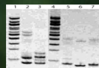
Fig.6. Example of electrophoreogram-10% PAGE. SSR analyses: 2-3 primers pair STM 1106 varieties Dali and Karin, 5-7 primers pair STWIN12C varieties Dali, Karin and Marabel, 1 and 4 DNA ladder marker 100 bp.
